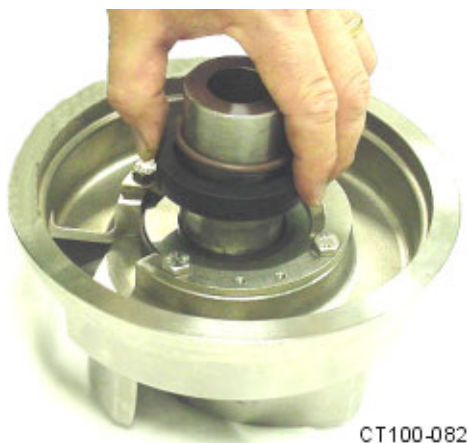
Figure 26 - Push Rotary Seal Down
