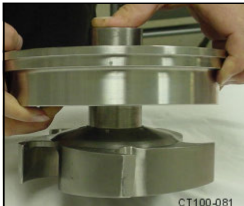
Figure 25 - Moving Rotary Seal Up the Shaft
