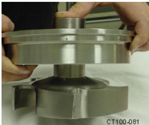
Figure 37 - Move Rotary Seal Up Shaft
