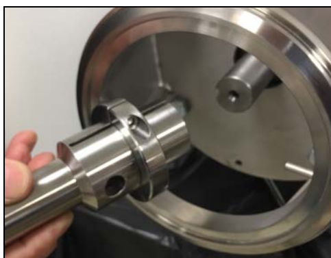
Figure 82 - Slide stub shaft on motor shaft
