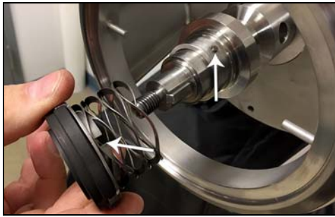
Figure 66 - Remove seal, cup, and spring
