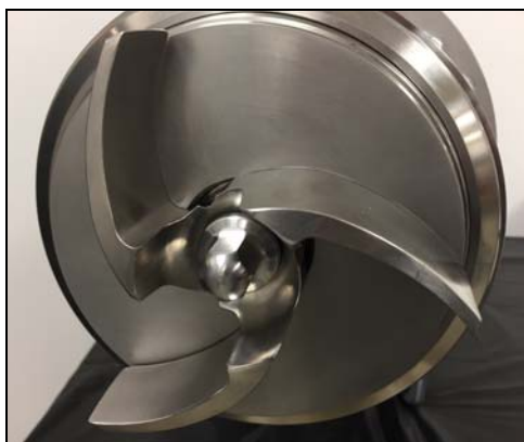
Figure 110 - Hand-tighten impeller nut
