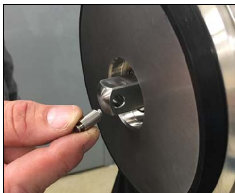
Figure 33 - Insert impeller retainer pin
