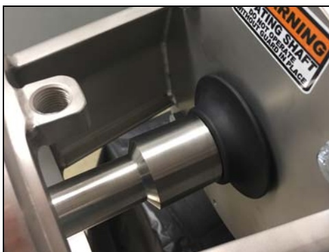
Figure 38 - Slide deflector onto shaft
