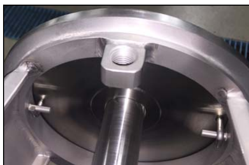
Figure 32 - Backplate pins engaged with adapter pins
