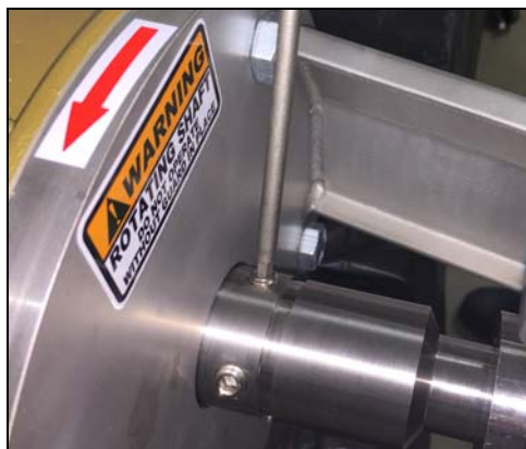
Figure 23 - Pin Impeller: Loosen setscrews
