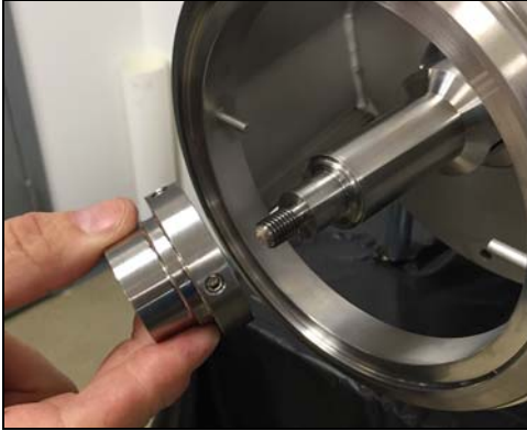
Figure 93 - Place drive collar on stub shaft
