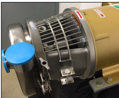
Figure 54 - Install guard assembly
