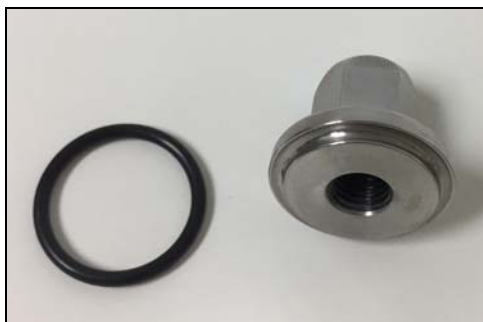
Figure 108 - Install O-ring on impeller nut
