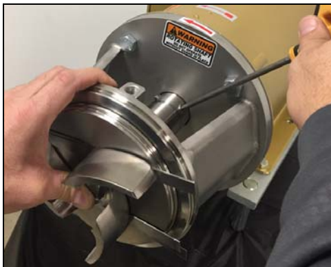
Figure 37 - Place feeler gauge, tighten setscrews
