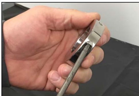
Figure 79 - Remove drive collar screws
