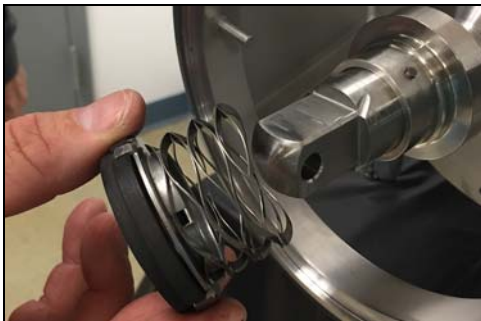
Figure 19 - Remove seal, O-ring, seal cup and spring
