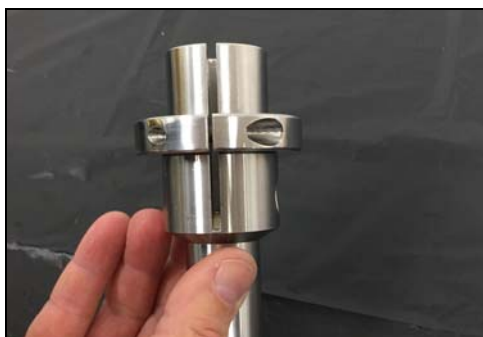
Figure 81 - Slide drive collar on stub shaft
