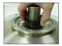
Figure 21 - Push Rotary Seal Down Releasing O-ring
