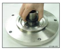
Figure 15 - Move Rotary Seal Up Shaft
