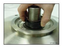
Figure 16 - Push Rotary Seal Down, Releasing O-ring
