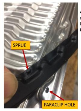
SPX FLOW / APV Heat Exchangers 1200 W. Ash Street Goldsboro, NC 27530 (888) 278-4321 As part of this product upgrade to a single piece end gasket, Paraclip elongated holes were added to the R5 end plates. The new end gasket is now provided with matching sprues to allow for the Paraclip of the plate and gasket.
