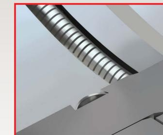
Used on seals that exceed the size and speed permitted for o-rings to center the sleeve on the shaft. The centering strip is fully captured in a dovetail groove.
