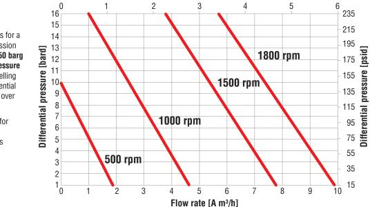
Performance curves for a typical gas transmission pipeline service at **50 barg** (725 psig) inlet pressure demonstrate compelling flow rate and differential pressure capability over various speeds.
