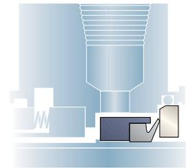
The Lip seal configuration features only one stationary component sealing radially against the rotating seal sleeve to contain the quench fluid.
