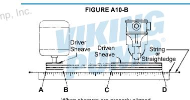
When sheaves are properly aligned, Mall points A, B, C, D will touch string or straightedge.
