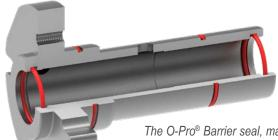
The O-Pro<sup>®</sup> Barrier seal, made of hardened cast iron, combines a bracket bushing and seal gland, with double O-ring seals, to stop process fluids from entering the bracket and eventually leaking from the pump.
