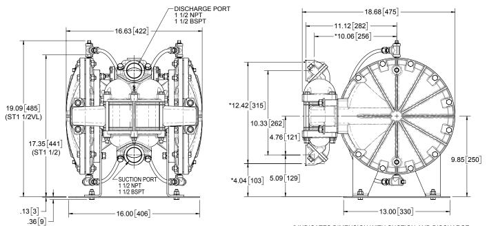
\* INDICATES DIMENSION WITH SUCTION AND DISCHARGE PORTS ROTATED 180° TO A VERTICAL POSITION
