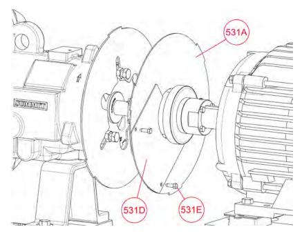
Figure 16-3: Motor End Plate
