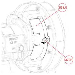
Figure 17-3: Bolt Guard into Place
