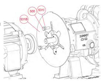
Figure 16-2: Pump End Plate
