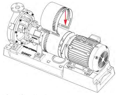
Figure 16-6: Second Shroud Install
