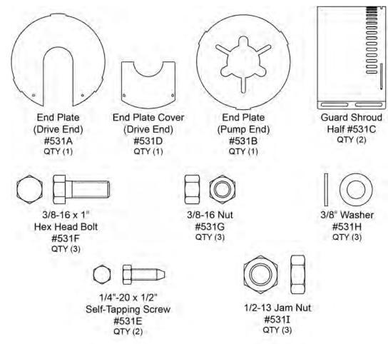
Figure 16-1: Barrel Coupling Guard Components
