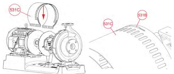
Figure 16-4: First Shroud Install
