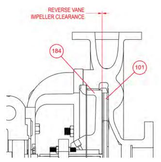
Figure 7-1: Reverse vane impeller clearance
