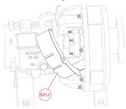
Figure 17-2: Fitting Adaptor Guard Half
