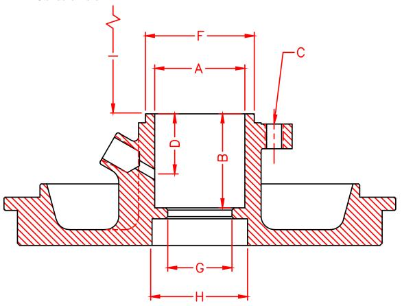
Figure 14-2: Standard Bore Stuffing Box Dimensions
