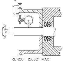
Figure 6-3: Measuring Runout
