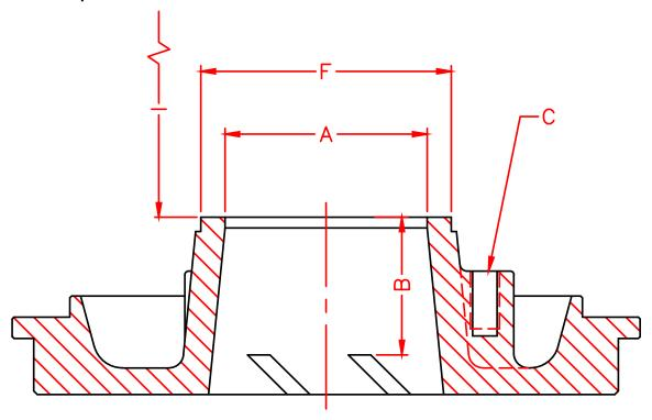
Figure 14-4: Taper Bore Stuffing Box
