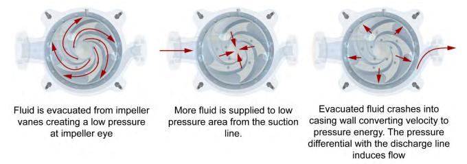
Figure 2-1: Basics of centrifugal design
