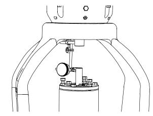
Figure 6-1: Fine Tune shaft alignment
