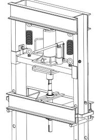
Figure 11-2: Setup for Removing Bearings
