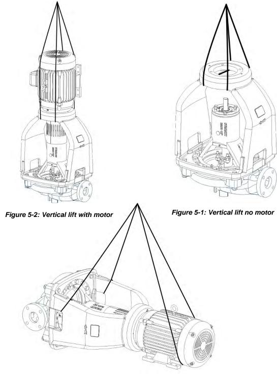
Figure 5-3: Horizontal Lift
