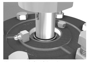
Figure 12-2: Lip Seal Orientation
