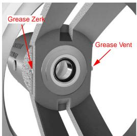
Figure 12-3: IB Lip Seal & Grease Fittings
