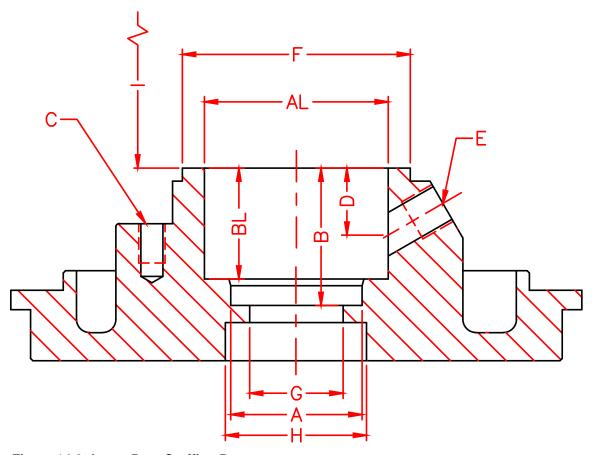
Figure 14-3: Large Bore Stuffing Box
