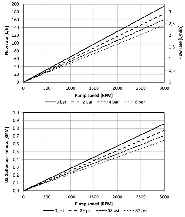
The flow rates showing at the chart above were ascertained with new diaphragms and new valves under standard conditions after the final assembly of the pump.
