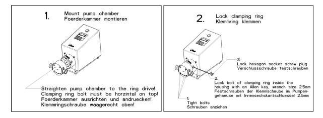
Pay attention to the following torque values: Image 2 item 1: Bolts pump chamber 4 Nm (3 lb-ft) Image 2 item 2: Bolt clamping ring 2 Nm (1.5 lb-ft)
