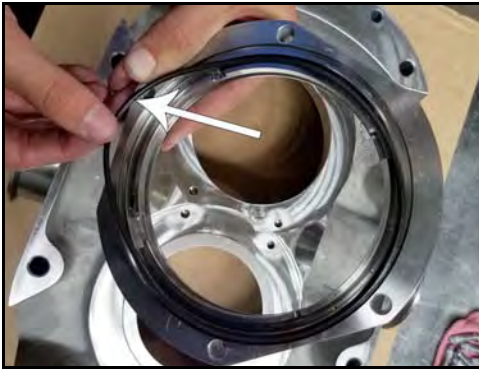
Figure 77 - Remove seal housing O-ring
