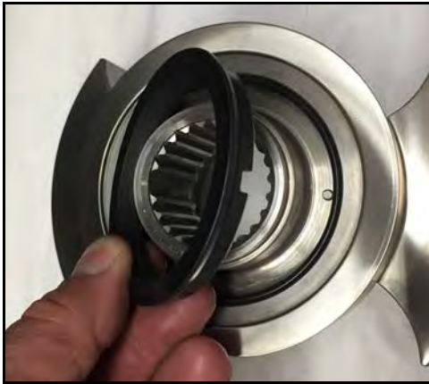
Figure 137 - Install rotary seal
