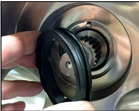
Figure 40 - Remove stationary seal
