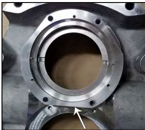
Figure 111 - Seal housing in place
