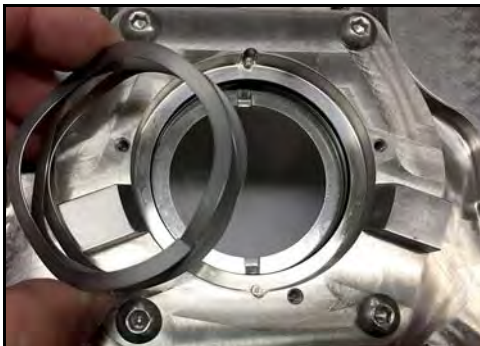
Figure 72 - Remove wave spring
