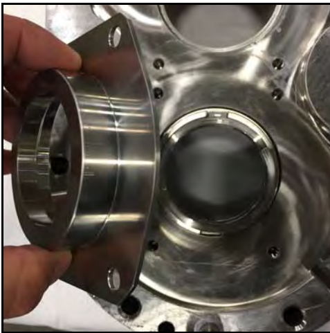
Figure 45 - Remove seal housing
