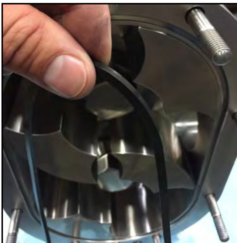
Figure 34 - Remove cover gasket
