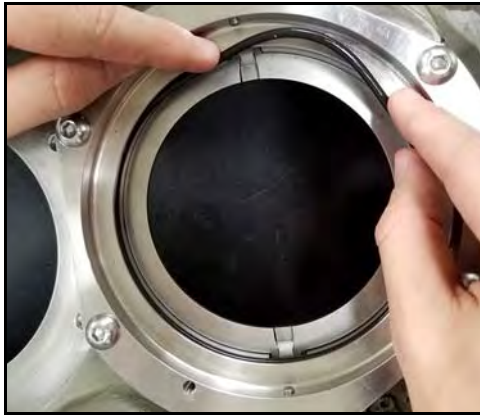
Figure 113 - Install seal O-ring
