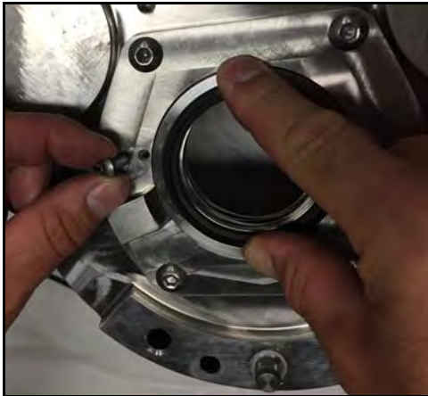
Figure 70 - Remove seal retaining bolts
