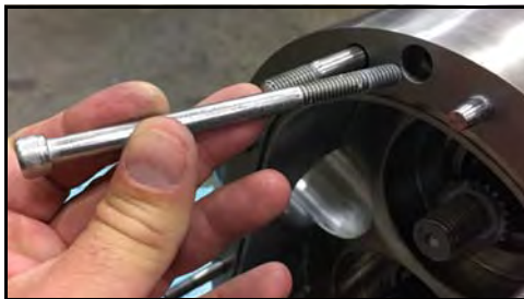
Figure 42 - Remove body retaining screws
