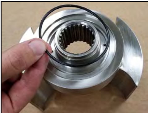
Figure 169 - Install sleeve front O-ring
