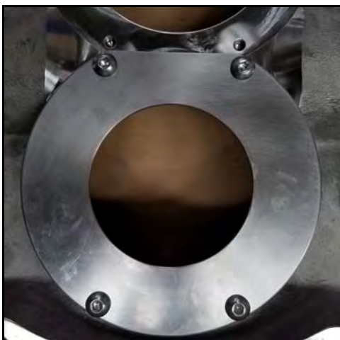
Figure 65 - Seal housing installed
