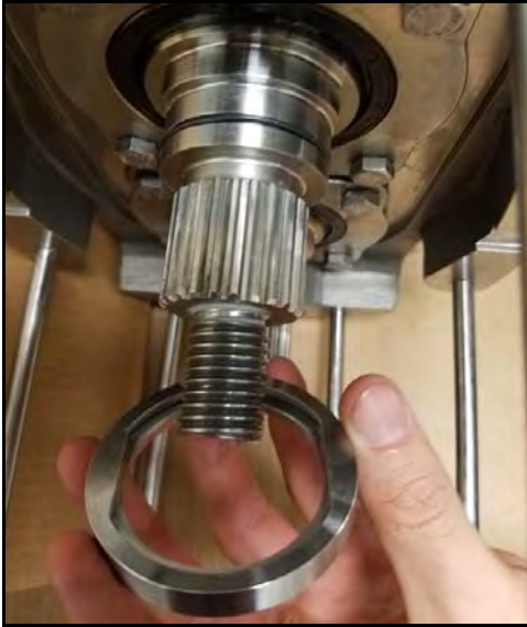
Figure 153 - Remove seal seat
