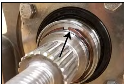
Figure 152 - Remove wave spring
