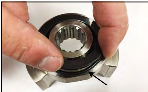
Figure 139 - Seal O-ring pinched
