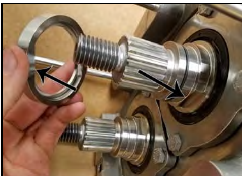
Figure 162 - Install seal seat
