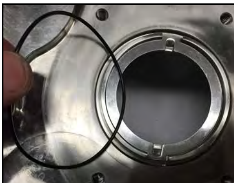
Figure 76 - Remove seal housing O-ring
