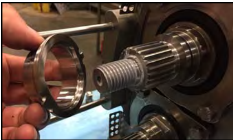
Figure 121 - Install adjusting ring
