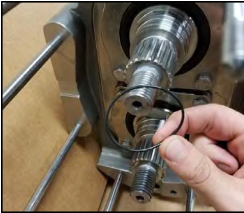
Figure 160 - Lubricate and install O-ring
