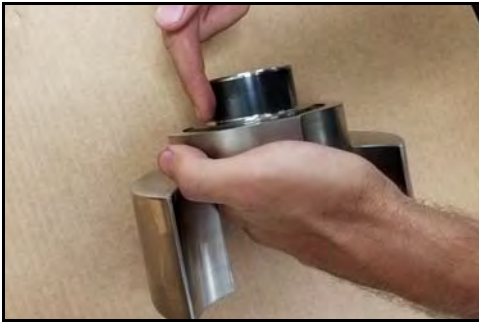
Figure 174 - Lubricate seal sleeve
