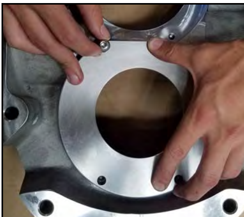
Figure 64 - Install seal housing bolts
