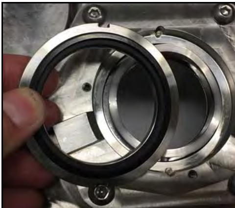
Figure 71 - Remove stationary seal
