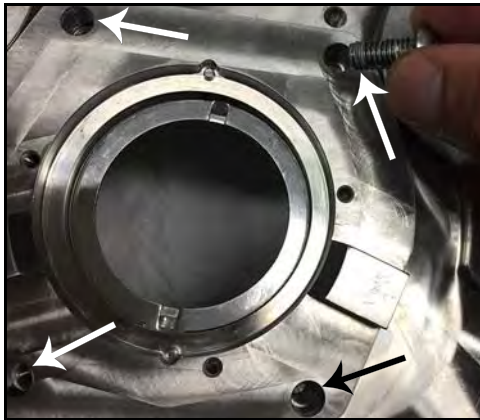
Figure 74 - Seal housing bolts
