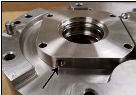
Figure 157 - Flush hole location
