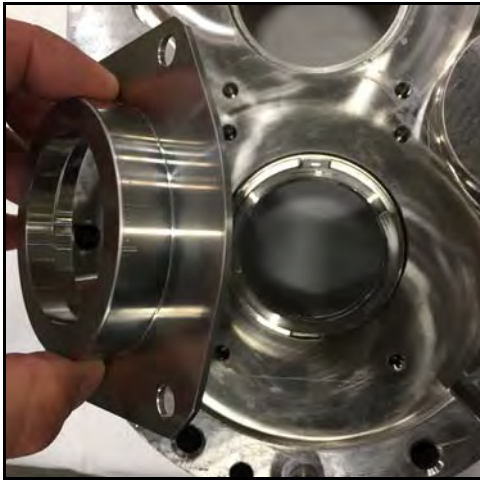
Figure 57 - Install seal housing
