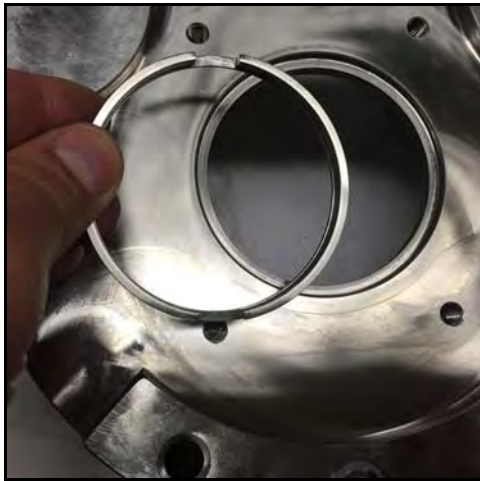
Figure 81 - Install shaft ring
