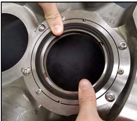
Figure 118 - Apply finger pressure
