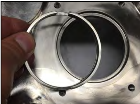
Figure 79 - Remove shaft ring
