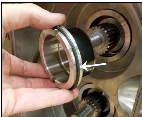
Figure 142 - Remove sleeve, O-ring
