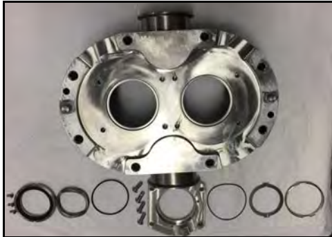
Figure 80 - Double Mechanical Seal (040-U3 shown)
