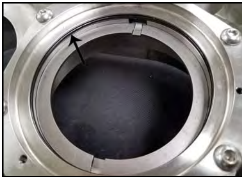
Figure 114 - Seal O-ring location
