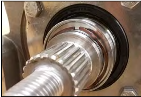
Figure 164 - Install wave spring
