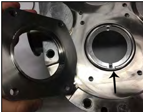
Figure 75 - Remove seal housing
