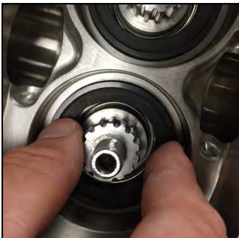
Figure 133 - Push on stationary seal
