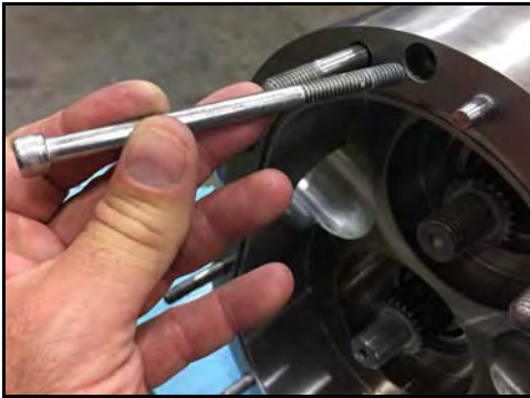
Figure 167 - Install body retaining screws
