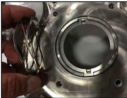
Figure 55 - Install wave spring
