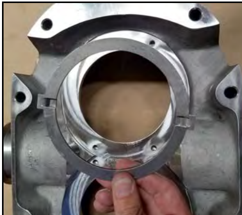
Figure 107 - Install drive ring
