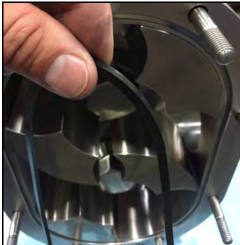
Figure 184 - Install cover gasket
