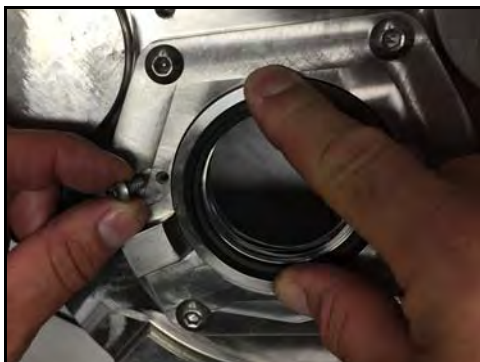
Figure 96 - Install seal retaining bolts
