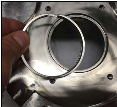
Figure 49 - Remove shaft ring
