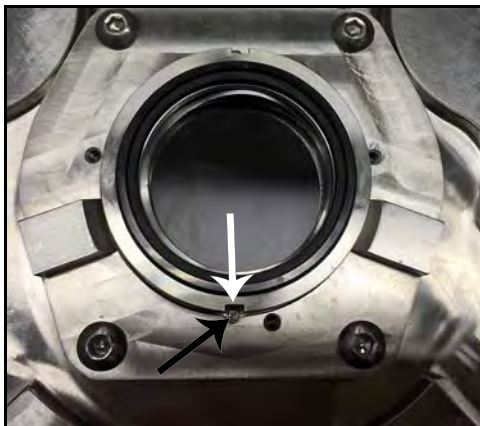
Figure 95 - Flush-side stationary seal installed
