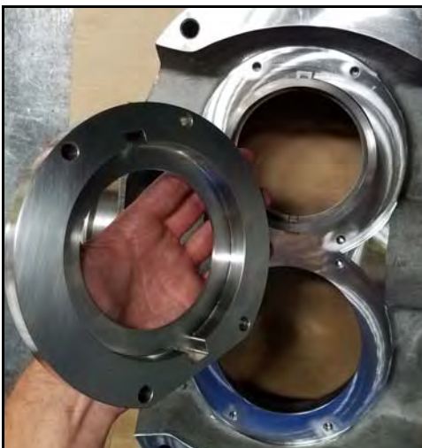
Figure 46 - Remove seal housing
