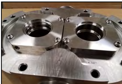
Figure 159 - Seal housings installed
