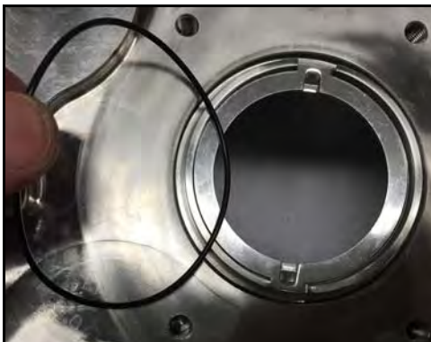
Figure 85 - Install seal housing O-ring
