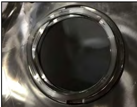
Figure 56 - Wave spring installed
