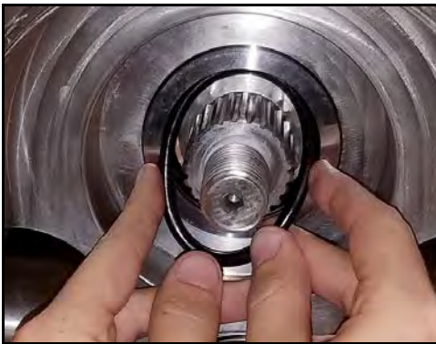
Figure 168 - Install seal O-ring
