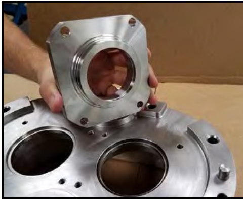
Figure 156 - Line up bolt holes
