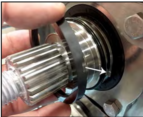
Figure 125 - Install flush-side rotary seal
