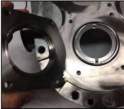
Figure 87 - Install seal housing
