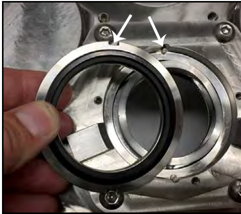
Figure 94 - Install flush-side stationary seal
