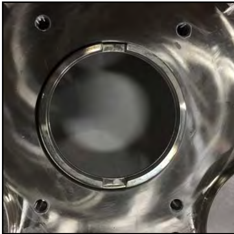
Figure 82 - Shaft ring installed
