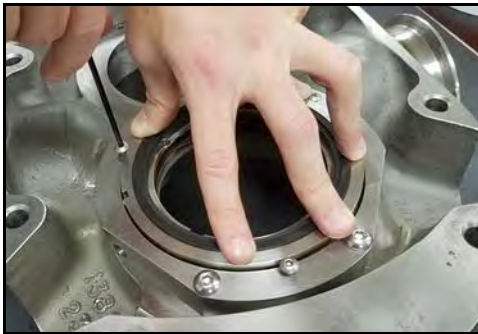
Figure 117 - Install seal retaining bolts
