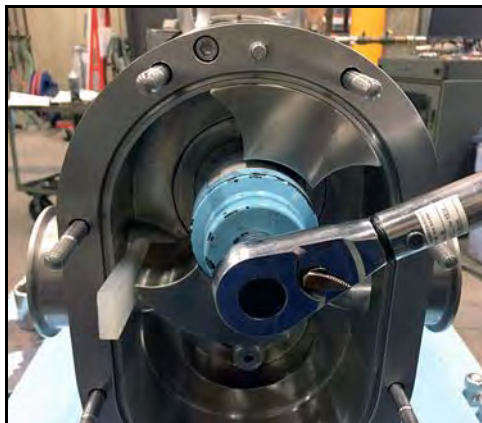
Figure 182 - Torque rotor nut
