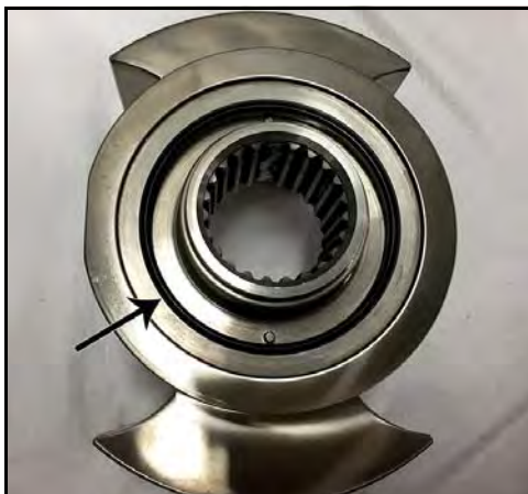
Figure 136 - Seal O-ring installed
