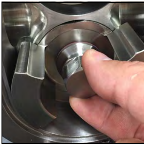
Figure 181 - Install rotor nut
