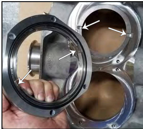
Figure 110 - Seal housing O-ring installed
