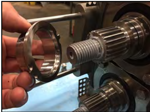
Figure 101 - Install adjusting ring
