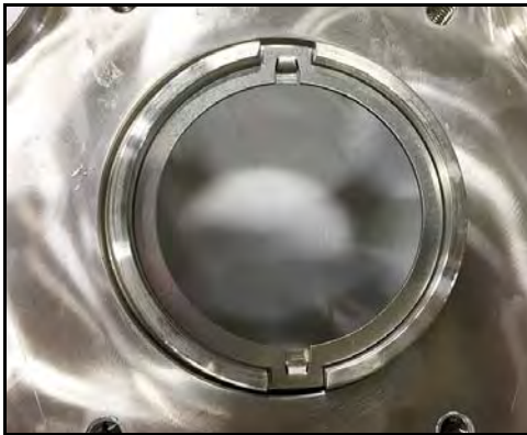
Figure 84 - Drive ring installed
