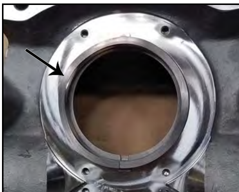
Figure 62 - Wave spring installed
