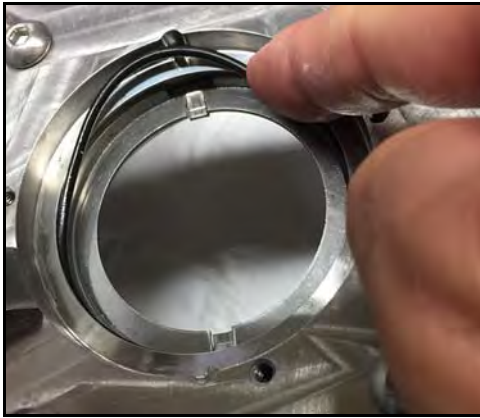
Figure 90 - Install seal O-ring
