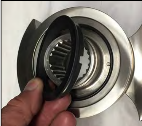
Figure 38 - Remove rotary seal
