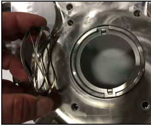
Figure 47 - Remove wave spring
