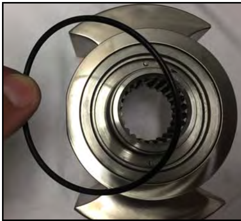
Figure 135 - Install seal O-ring
