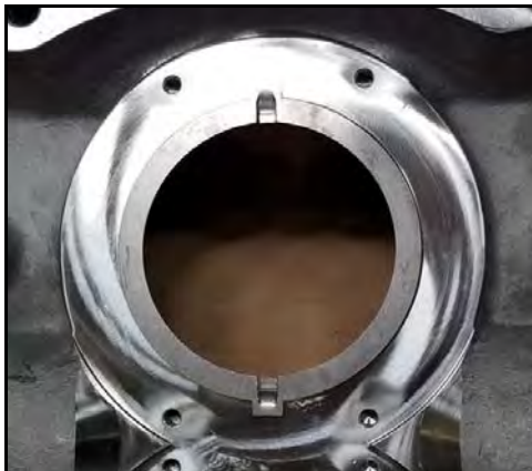
Figure 61 - Drive ring installed
