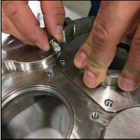
Figure 44 - Remove seal housing bolts
