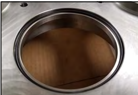
Figure 155 - Seal housing O-ring installed
