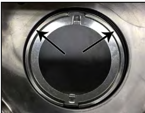
Figure 86 - Seal housing O-ring installed
