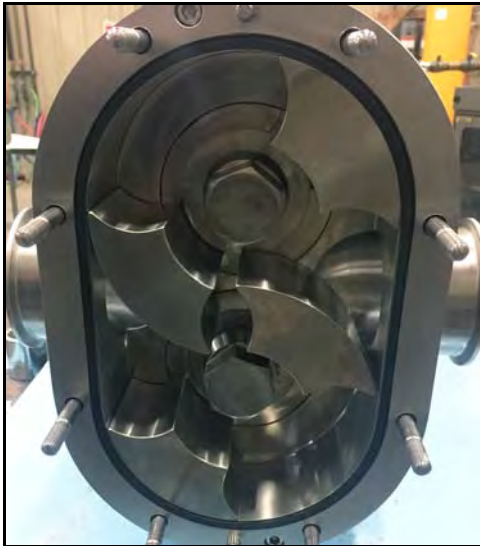
Figure 185 - Cover gasket installed
