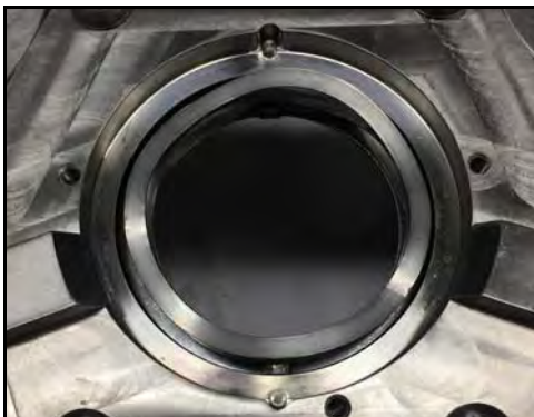
Figure 93 - Wave spring installed
