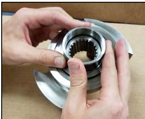
Figure 172 - Press sleeve into place
