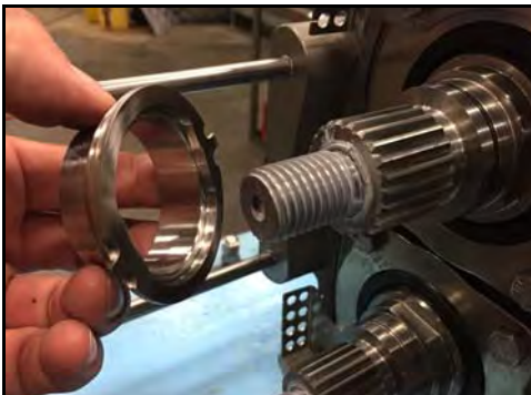
Figure 68 - Remove adjusting ring
