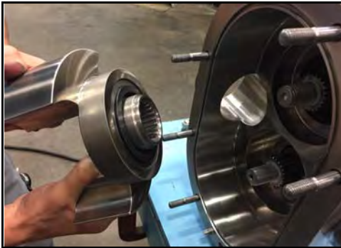
Figure 177 - Push rotor on shaft
