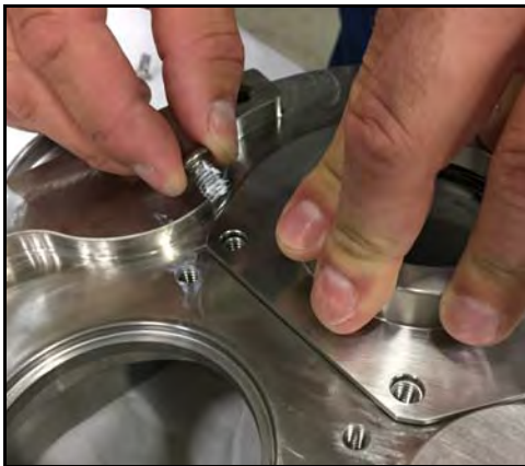
Figure 58 - Install seal housing bolts
