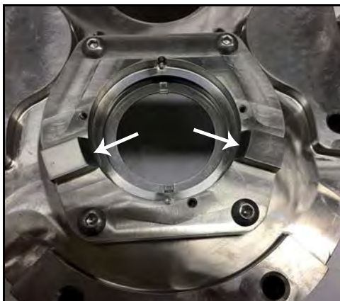
Figure 89 - Seal housing installed
