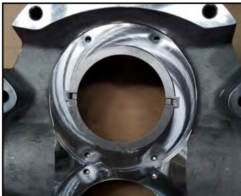
Figure 108 - Drive ring installed
