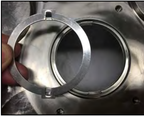
Figure 83 - Install drive ring
