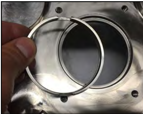
Figure 51 - Install shaft ring
