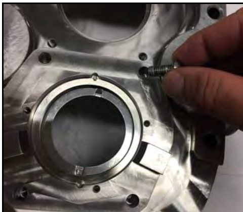
Figure 88 - Seal housing bolts
