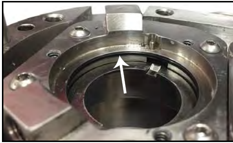
Figure 73 - Seal O-ring location
