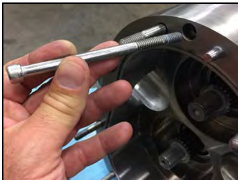
Figure 129 - Install body retaining screws
