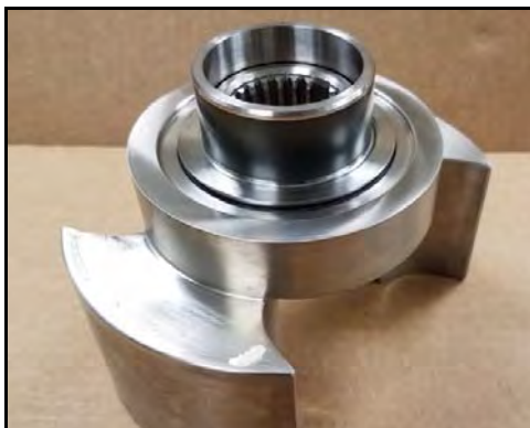
Figure 173 - Seal sleeve installed
