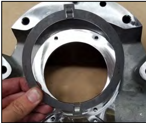
Figure 60 - Install drive ring
