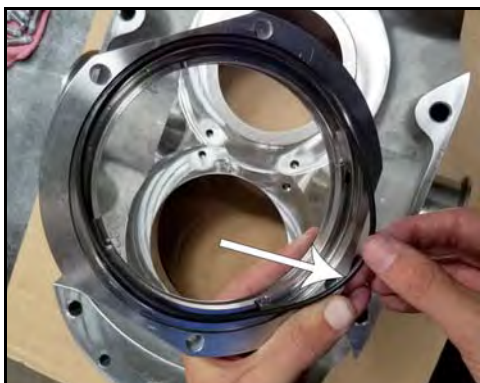
Figure 109 - Install seal housing O-ring
