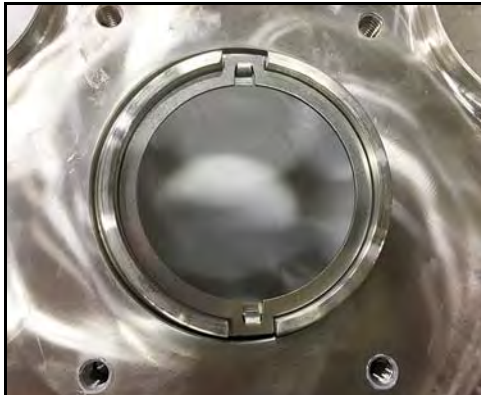
Figure 54 - drive ring installed (130-U3 and smaller)
