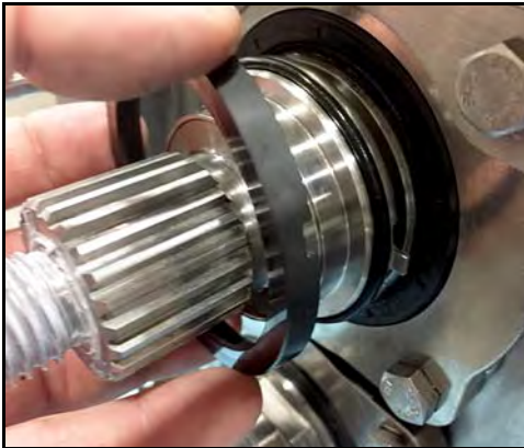
Figure 66 - Remove flush-side rotary seal
