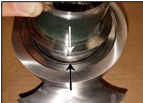
Figure 171 - Line up notch and pin
