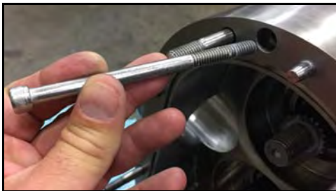
Figure 147 - Remove body retaining screws
