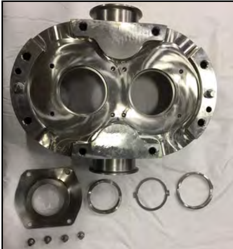
Figure 50 - Single Mechanical Seal (040-U3 shown)
