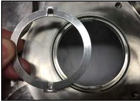
Figure 53 - Install drive ring
