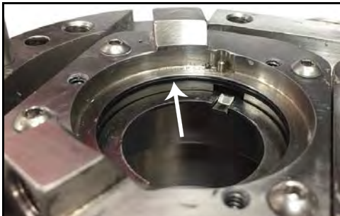
Figure 91 - Seal O-ring location
