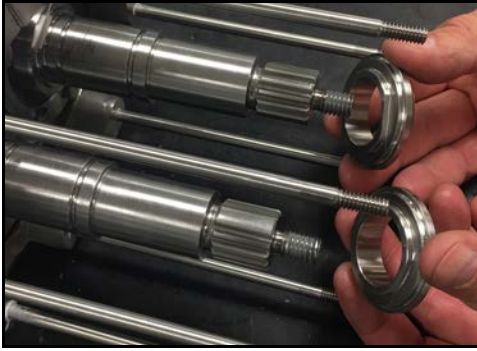
Figure 204 - Install seal caps
