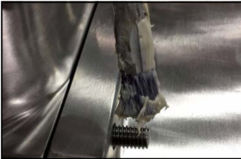
Figure 120 - Apply anti-seize to threads
