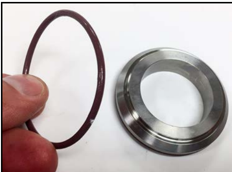
Figure 39 - Remove cap-to-screw O-ring
