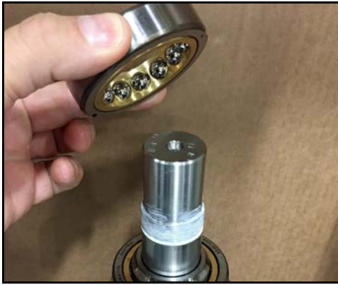
Figure 159 - Place bearing onto race
