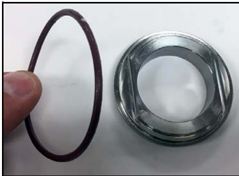
Figure 91 - Install cap-to-seat O-ring
