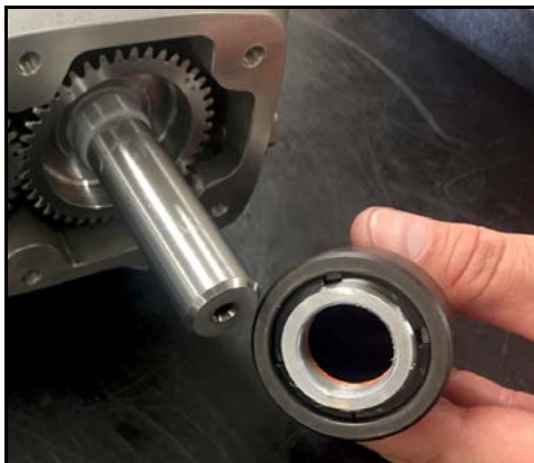
Figure 131 - Remove locking nut and gear
