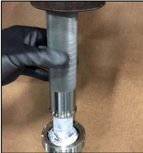
Figure 152 - Press race onto shaft
