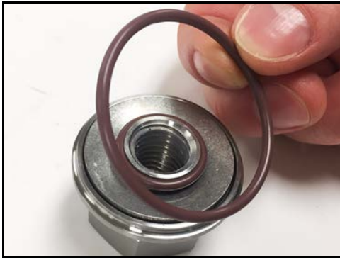
Figure 110 - Install screw nut O-ring
