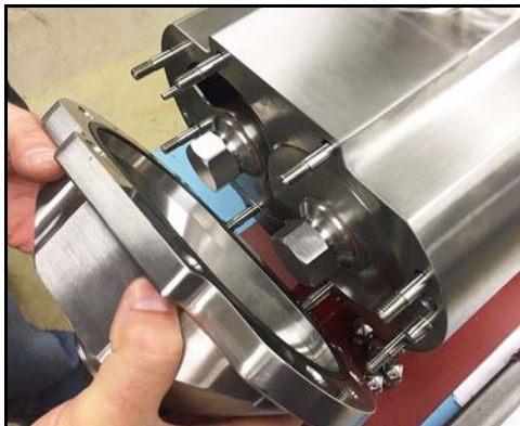
Figure 28 - Remove pump cover
