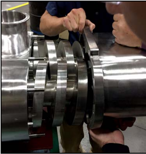
Figure 118 - 220-UTS Install pump cover
