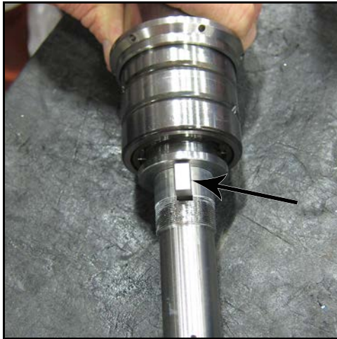
Figure 170 - Place key in keyway
