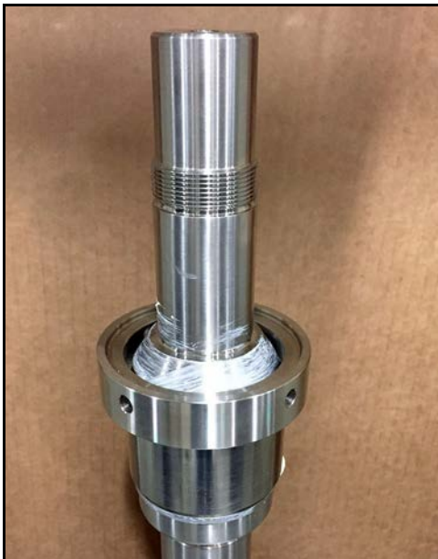
Figure 147 - Bearing spacer installed
