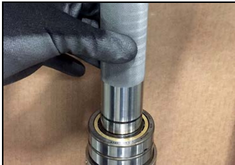
Figure 165 - Press race onto shaft
