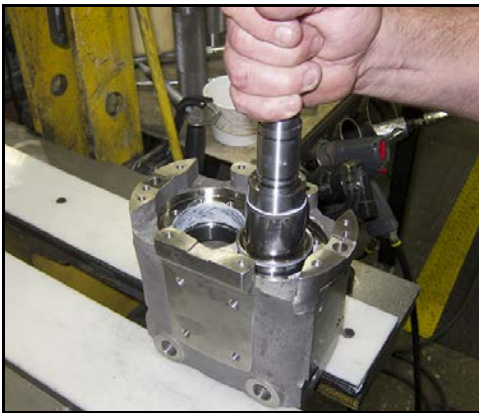
Figure 175 - Place short shaft in bore
