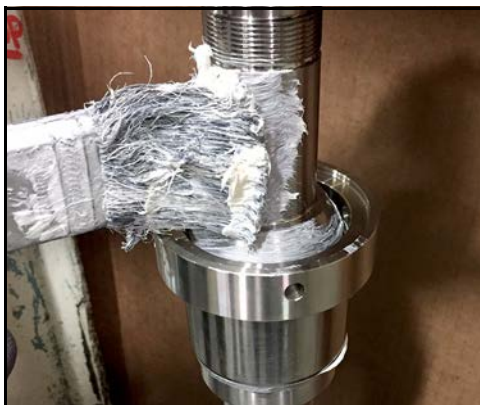
Figure 150 - Apply anti-seize to shaft
