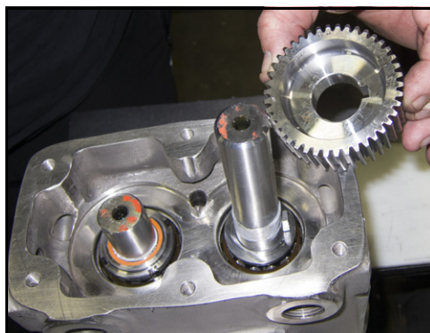
Figure 191 - Install drive gear
