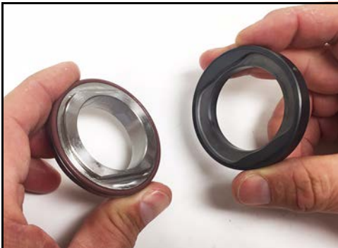
Figure 38 - Remove seal seat from seal cap
