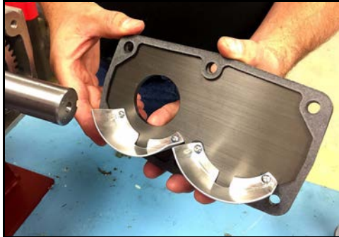
Figure 222 - Place gasket on cover
