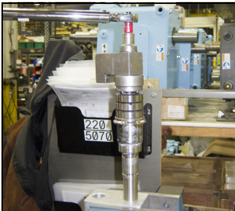
Figure 168 - Torque down locking nut
