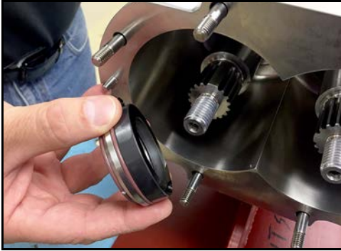
Figure 37 - Remove seal cap assembly
