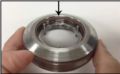
Figure 64 - Carrier-to-seal O-ring installed
