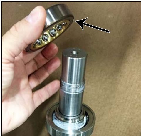
Figure 154 - Place bearing onto race
