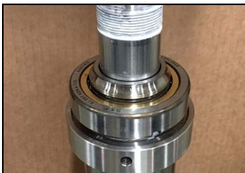
Figure 158 - Press race into bearing
