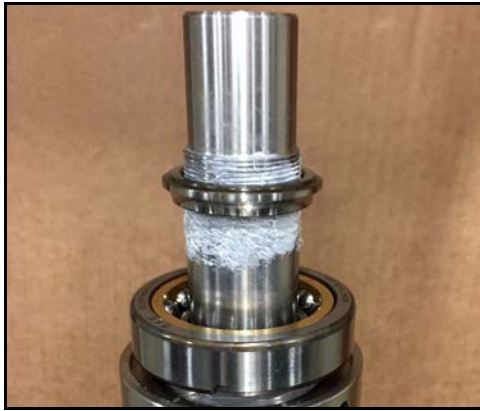
Figure 155 - Place race on shaft
