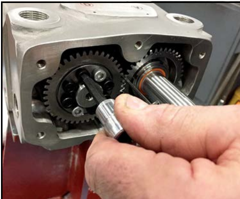
Figure 214 - Hand-tighten locking assembly bolts
