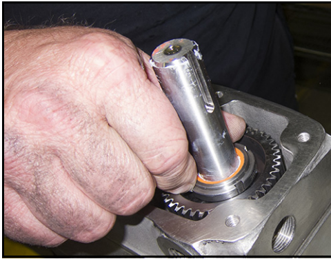
Figure 194 - Install locking nut
