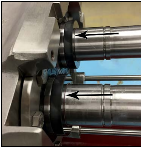
Figure 80 - Seal seats installed
