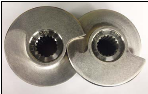
Figure 101 - Arrange screws: LH-RH
