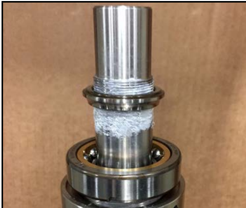
Figure 160 - Place race on shaft
