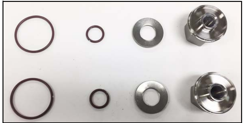
Figure 106 - Screw Nut Components
