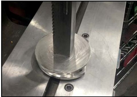
Figure 183 - Install bearing retainer seal
