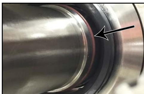
Figure 85 - Install shaft O-ring
