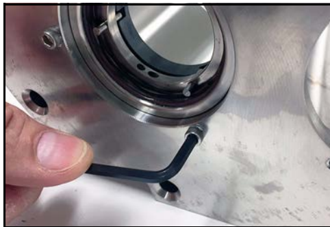
Figure 50 - Remove cap screws
