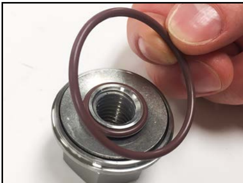
Figure 32 - Remove screw nut O-ring
