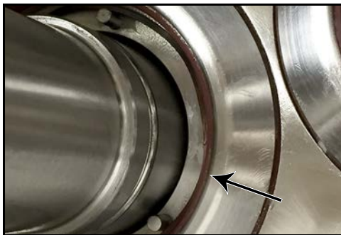
Figure 43 - Remove carrier-to-seal O-ring
