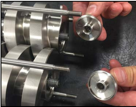
Figure 206 - Install screw nuts
