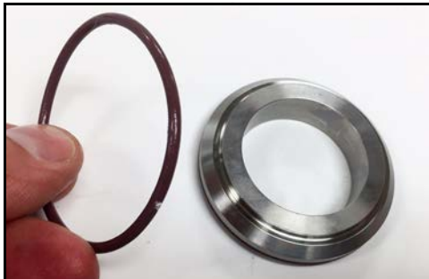
Figure 93 - Install cap-to-screw O-ring
