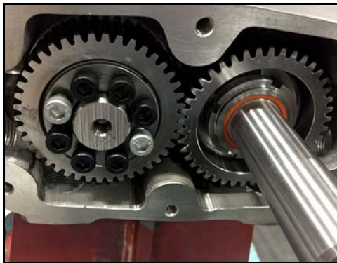
Figure 203 - Align loose gear with drive gear
