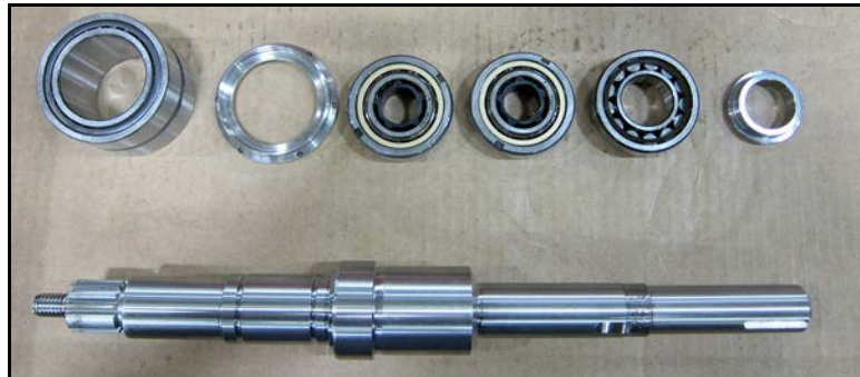
Figure 139 - Drive Shaft: Assembly items needed
