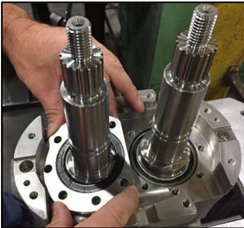
Figure 133 - Remove bearing retainer
