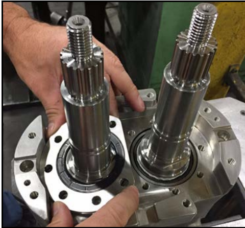
Figure 188 - Install bearing retainer
