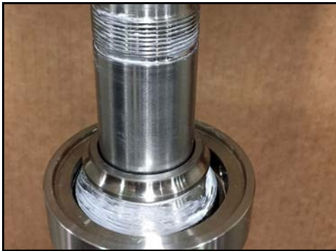
Figure 153 - Race pressed on shaft
