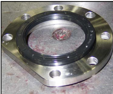
Figure 182 - Center bearing retainer seal
