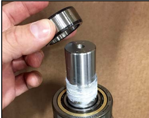
Figure 164 - Place race onto shaft
