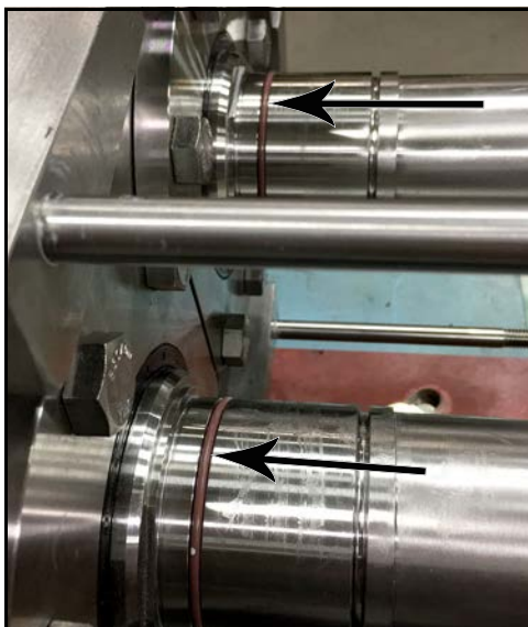
Figure 78 - Install shaft O-rings
