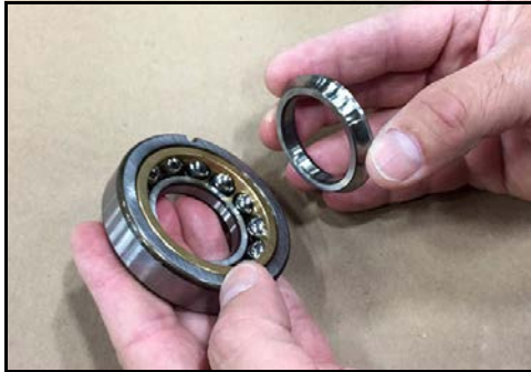
Figure 149 - Remove bottom race
