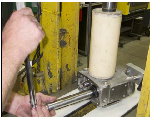
Figure 196 - Torque locking nut
