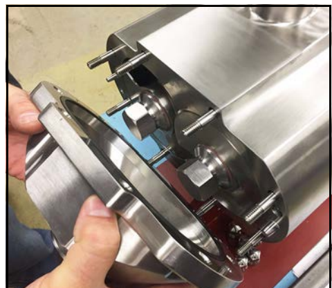
Figure 117 - Install pump cover
