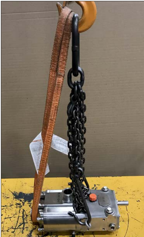
Figure 1 - Lifting location - 015, 030-UTS
