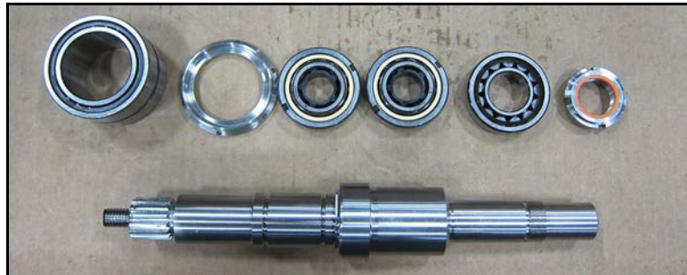
Figure 140 - Short Shaft: Assembly items needed
