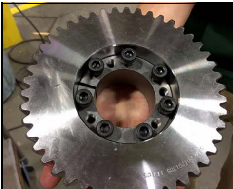
Figure 201 - Place locking assembly into gear
