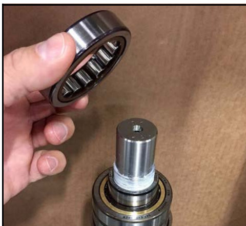
Figure 166 - Place bearing onto race
