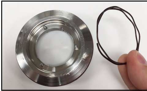
Figure 54 - Seal wave spring
