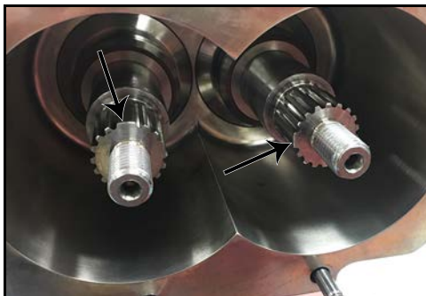
Figure 102 - Align screw and shaft spline
