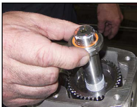
Figure 193 - Install locking nut
