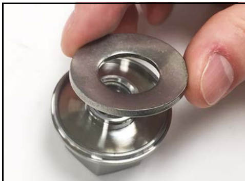
Figure 107 - Install belleville washer
