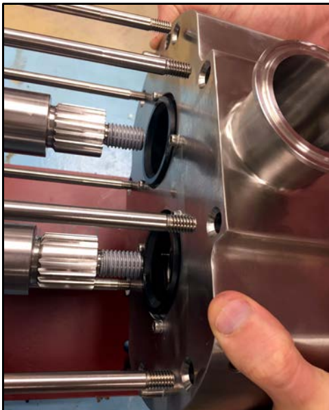
Figure 81 - Install pump body onto shafts
