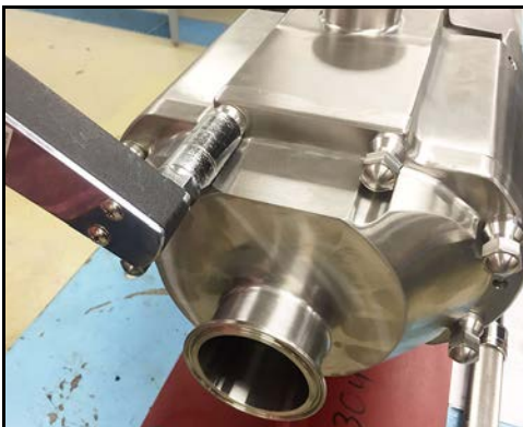
Figure 121 - Torque cover nuts
