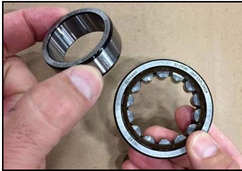
Figure 163 - Remove race from bearing
