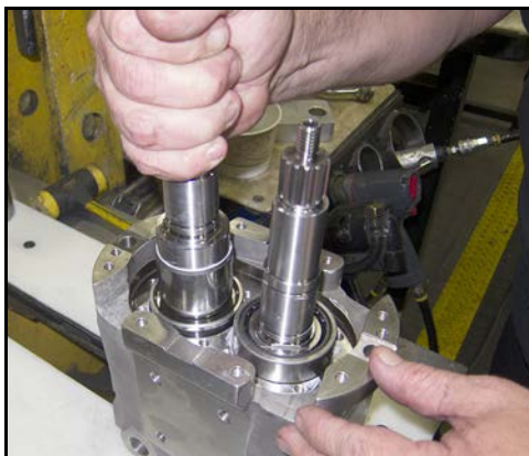
Figure 178 - Place drive shaft in bore
