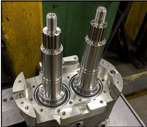
Figure 181 - Shafts seated in gearcase
