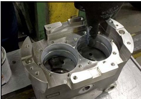
Figure 174 - Spread even layer
