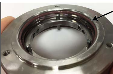
Figure 66 - Carrier-to-seal O-ring installed
