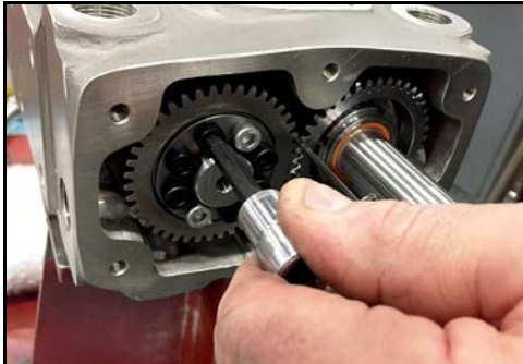
Figure 126 - Loosen bolts in locking assembly
