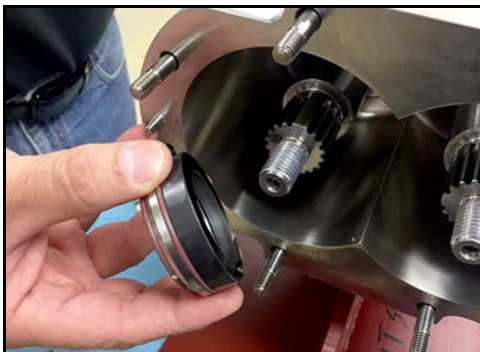
Figure 97 - Install seal cap assembly
