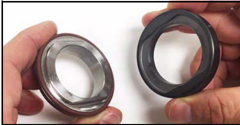
Figure 95 - Line up seal cap and seal seat
