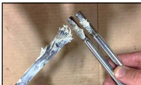
Figure 83 - Apply anti-seize to threads
