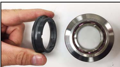
Figure 67 - Lubricate and install seal
