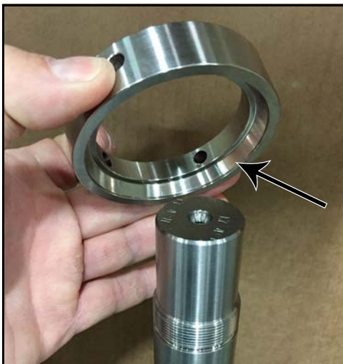
Figure 146 - Place bearing spacer on shaft
