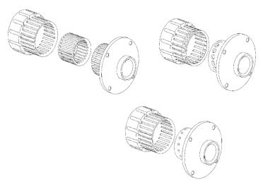
Interchange modular stators and rotors to achieve desired effect.
